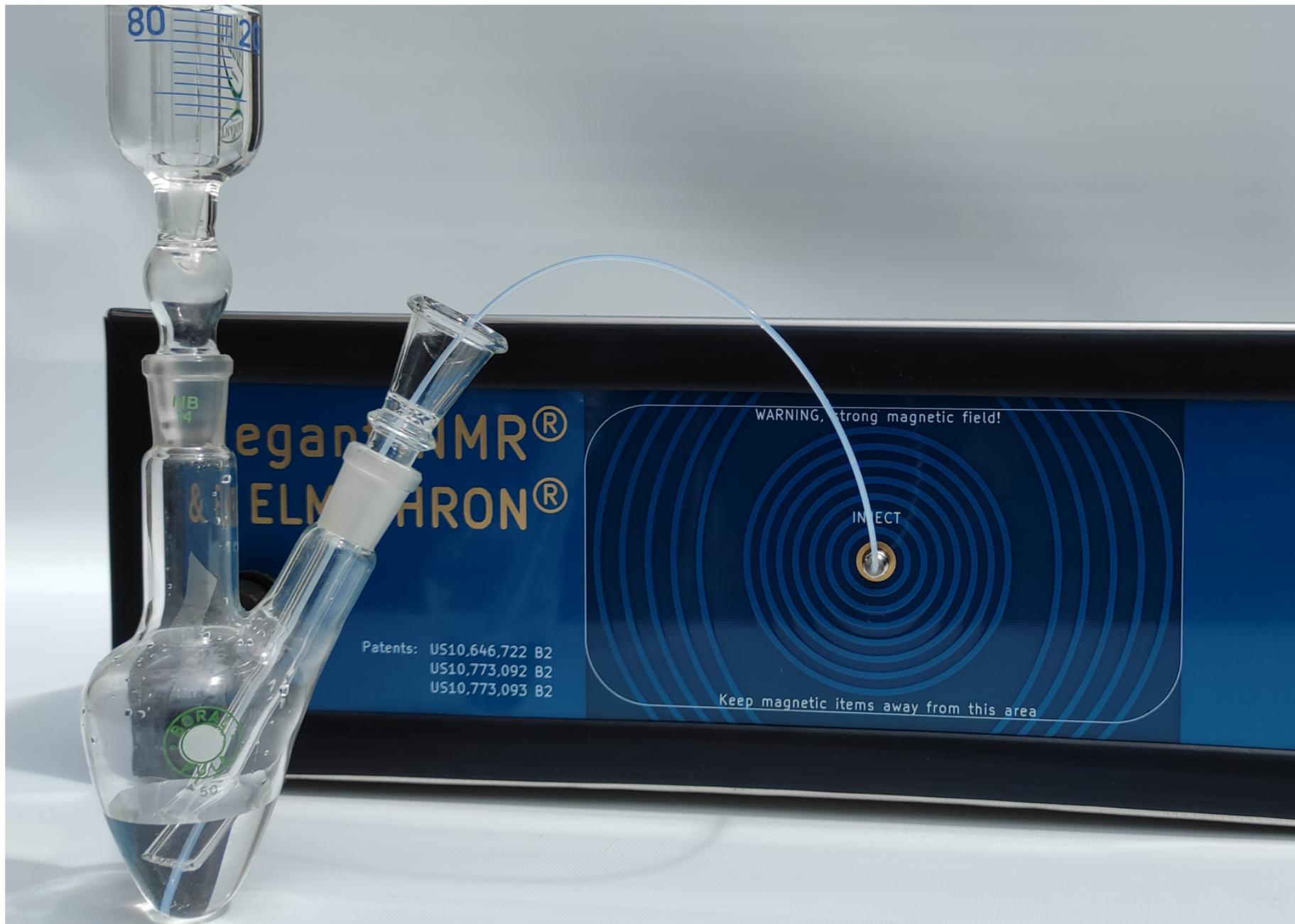
You must turn on Elmathron, connect a vacuum, start up the device, connect a capillary to the inlet and place the inlet capillary in the liquid to be measured.
